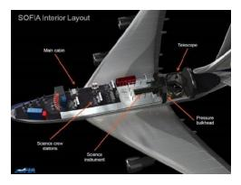
Built within the frame of a Boeing 747SP, SOFIA contains an internally mounted 2.7-meter (approximately 9-foot) telescope that operators expose to the night sky through a uniquely designed cavity door located at the rear of the plane. NASA designed SOFIA to observe both infrared and visible wavelengths from 0.3 to 1.600 microns.
